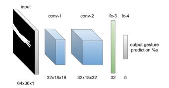
Fig. 5. Extracted and downsized hand gesture depth images underwent two convolutional layers and two fully connected layers, with the last layer serving as a softmax classifier.
