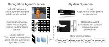
Fig. 1. Overall system workflow consists of two separate processes: (left) creating gesture recognition agent (right) implementing real-time classification of real-world gestures
