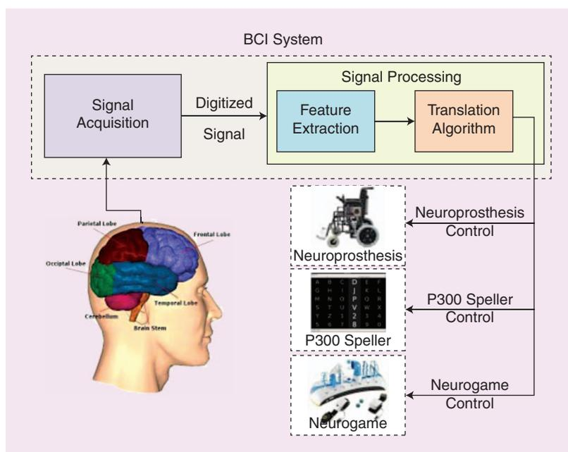
**FIGURE 1.** High-level block diagram of a typical brain-computer interface.
