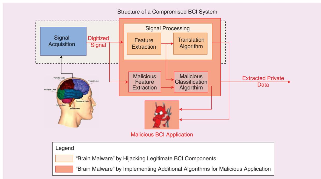
**FIGURE 2.** A simplified diagram of a compromised BCI system. We distinguish between two types of attackers: a) an attacker who exploits the legitimate feature extraction and decoding (translation) algorithms (denoted as orange blocks in the diagram), and b) an attacker who implements an additional malicious application, and either replaces or supplements the legitimate BCI resources (denoted as red blocks in the diagram).
